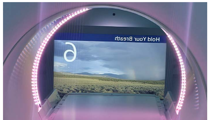
Countdown Timer and Scrolling Text Features to help with breath hold management
