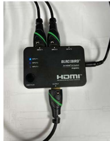
**STEP 2.5:** If there are other HDMI-compatible video sources the customer wishes to add, connect an HDMI from the video source to an available HDMI Switch Input
