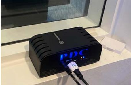
2. **Wireless Receiver/Transmitter (RxTx)** – Installed on the RF window ledge in the **Scan room**
