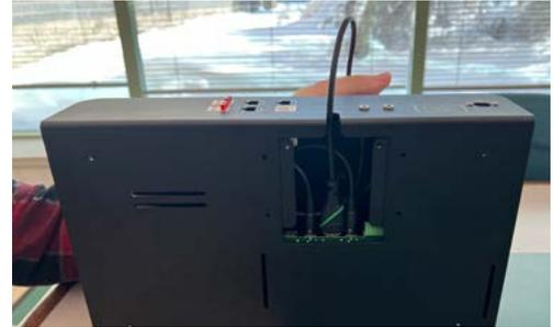
**STEP 2.3:** Close up back access panel on the AVC (note: slide in bottom lip of panel first when placing back on box)
