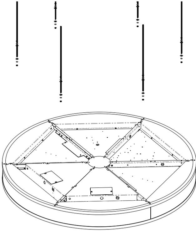
Diagram 3 - Threaded Rod Mount Detail
