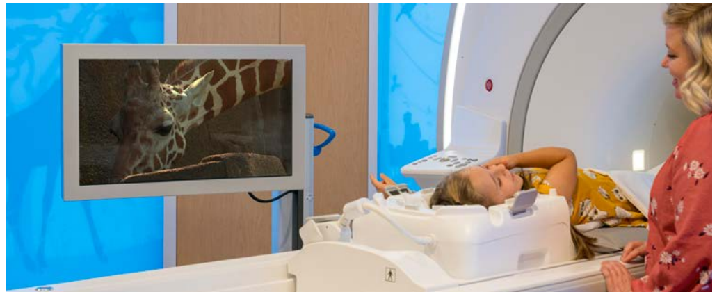
Feet-First Scan - MRI Wireless Portable Video Display can be placed next to the patient or behind the bore
